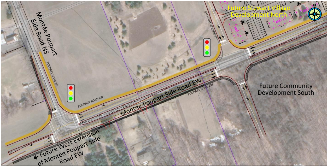
Figure 5-6: Intersection No. 3 & No. 4: Traffic Signal Controlled Alternative
